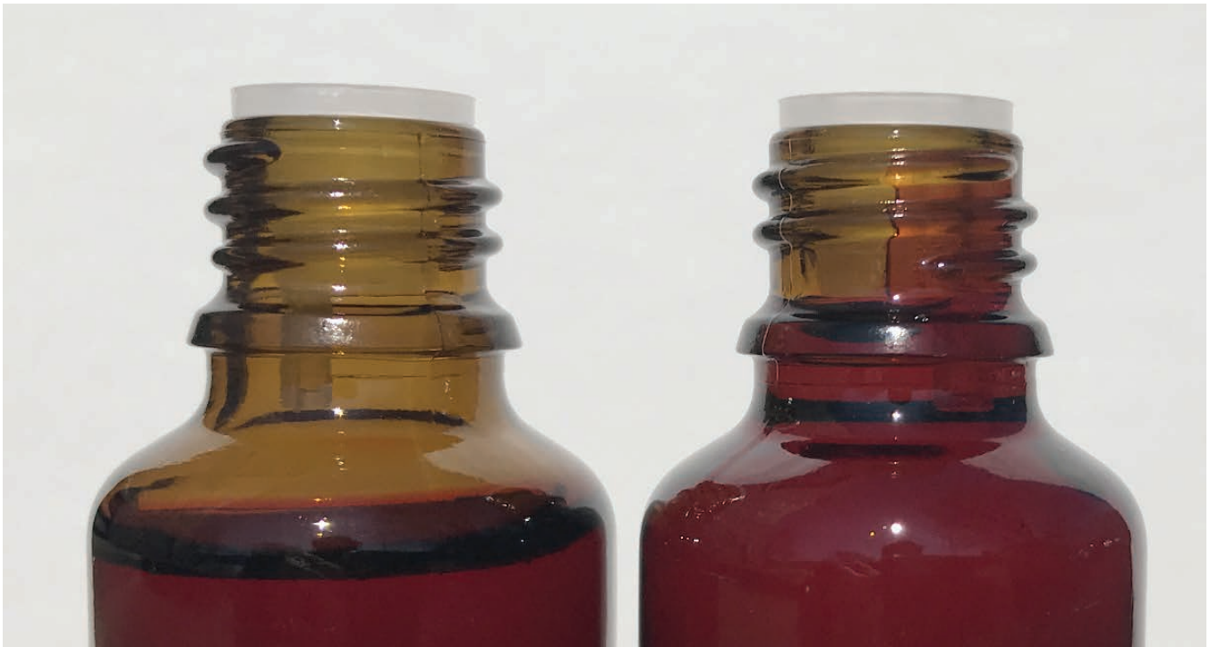
Bottle on left shows proper fill with meniscus of liquid at shoulder level. Bottle on right shows overfill with liquid covering the Dropper Insert. This will cause leakage onto the neck and result in the cap backing off during shipping and storage.
